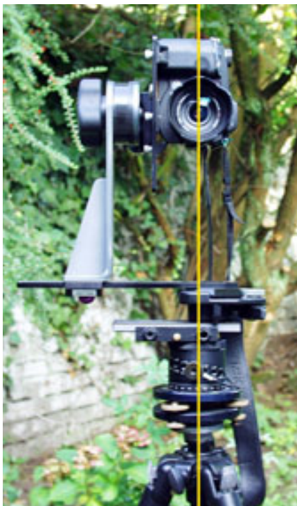
The centre of the lens and the rotating axis are on a same vertical line.
