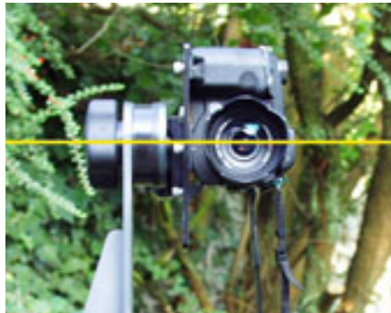
The centre of the lens and the tilting axis are on a same horizontal line.
